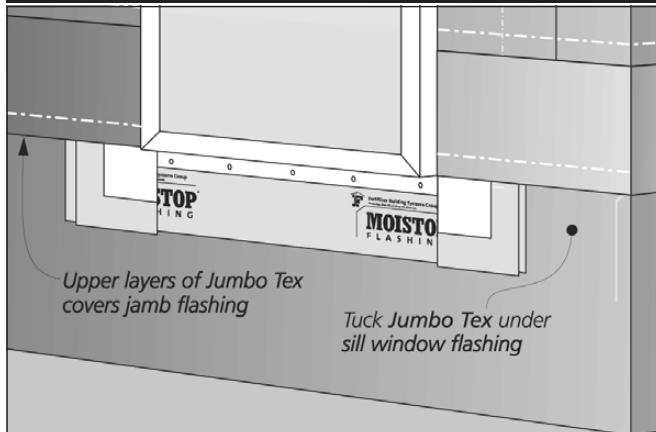
When a layer of **Jumbo Tex** first crosses the path of any window, it needs to be properly integrated with the window sill and jamb flashing for quality moisture management. To do this, tuck **Jumbo Tex** under the sill and jamb flashing as shown above. The layers above this point can butt into the window jamb.
