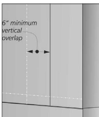
At vertical seams, apply a minimum 6" vertical overlap. When going around corners, make sure **Jumbo Tex** is pulled tightly and properly fastened.
