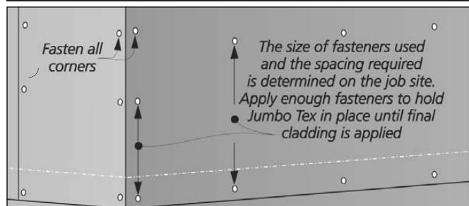
Under normal conditions, attaching **Jumbo Tex** with a quality exterior grade staple is acceptable. A higher grade of galvanized fastener, or large headed galvanized nail may be required in certain settings or weather conditions.
