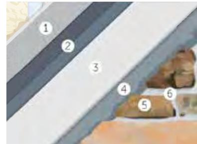
In sequence: (1) sheathing, (2) two layers of water resistant barrier (WRB), (3) cement board, (4) mortar setting bed, (5) Cultured Stone manufactured stone veneer, (6) mortar joint.
