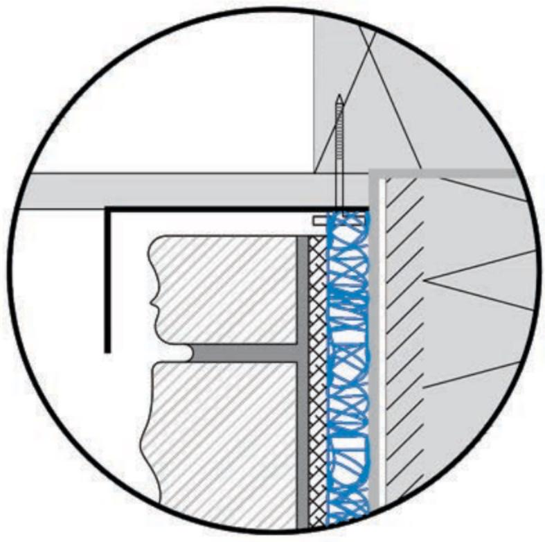
Be mindful of differential movement when the flashing is attached directly to the soffit.
