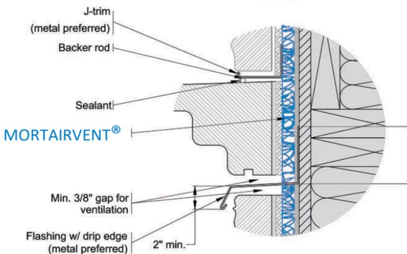
MANUFACTURED STONE TO MANUFACTURED STONE TYPICAL TRANSITION
