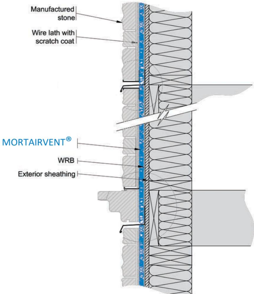
MANUFACTURED STONE TO MANUFACTURED STONE TYPICAL TRANSITION
