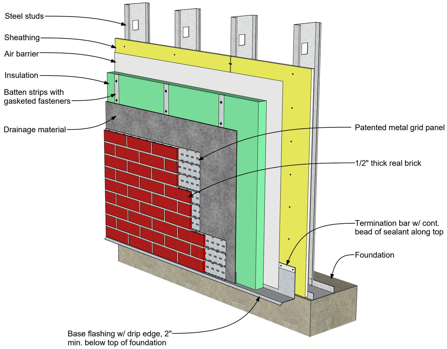
CIS Exterior Wall, Steel Stud Backing | Base of Wall
