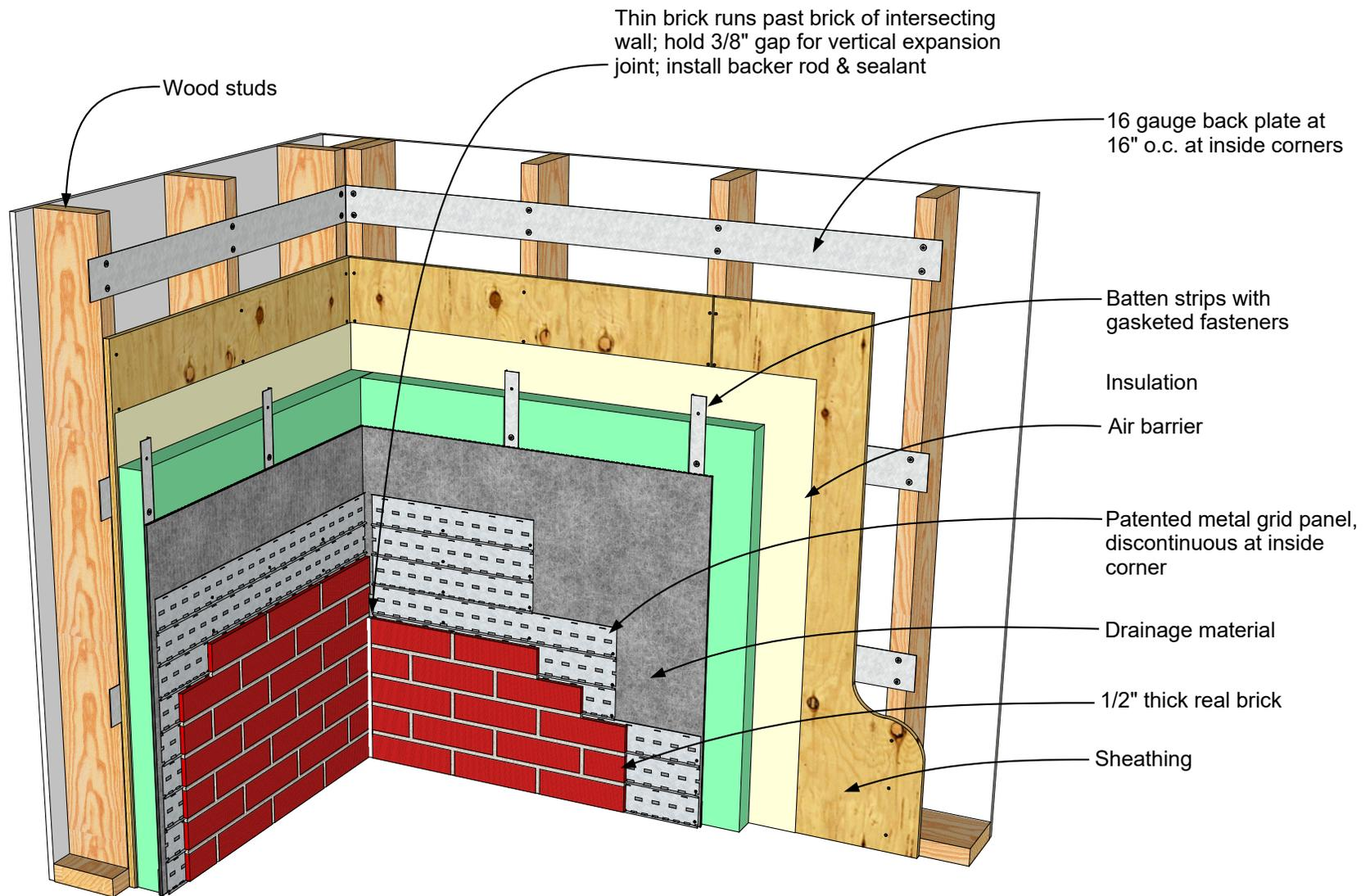
CIS Exterior Wall, Wood Stud Backing | Inside Corner
