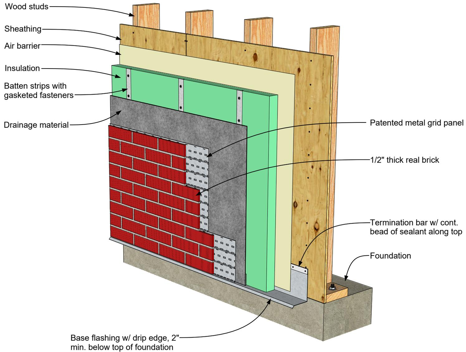
CIS Exterior Wall, Wood Stud Backing | Base of Wall
