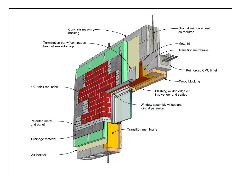
CIS Exterior Wall, CMU Backing | Window Head Detail 05.01.03 Rev. 12/28/18
