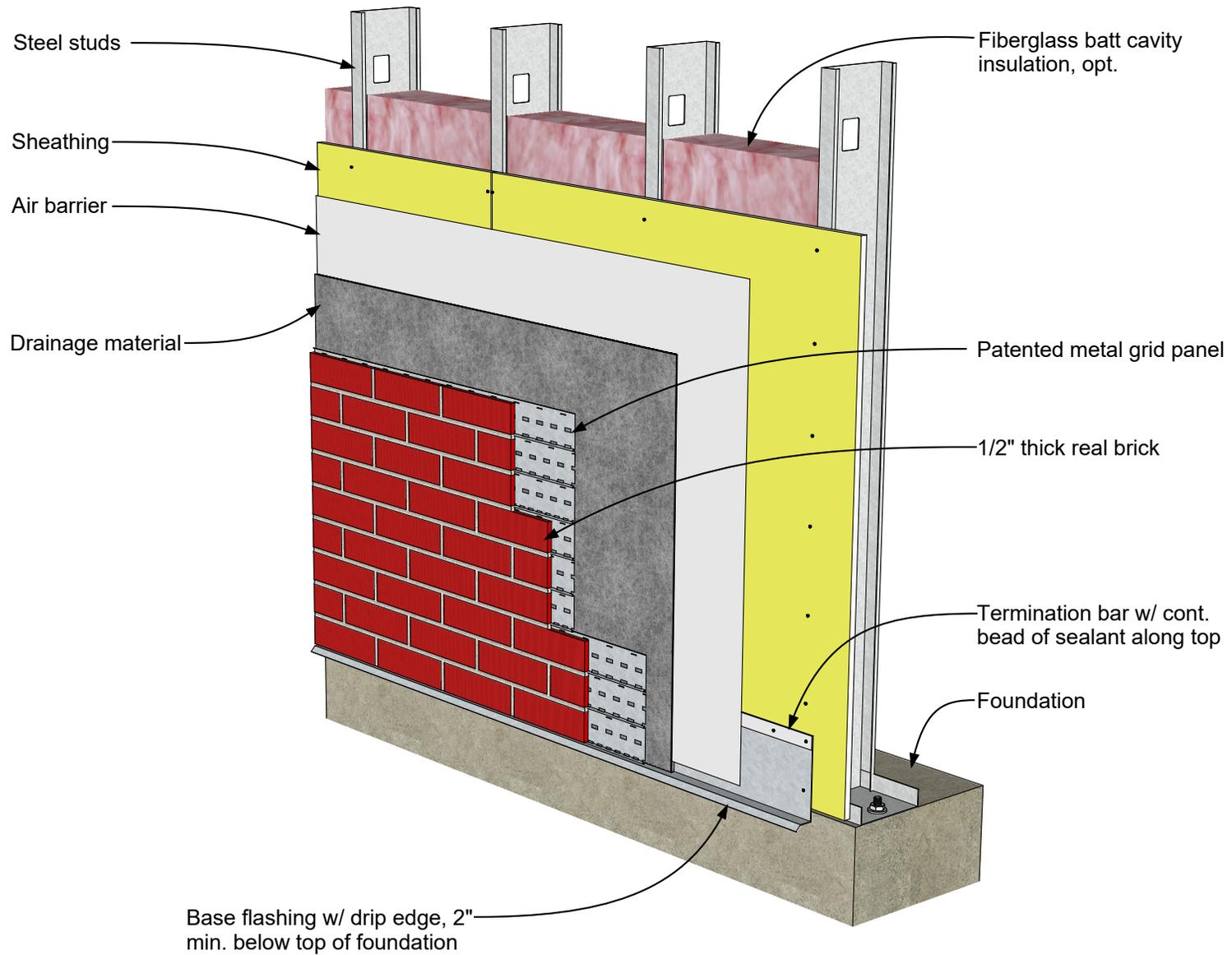
MCS Exterior Wall, Steel Stud Backing | Base of Wall
