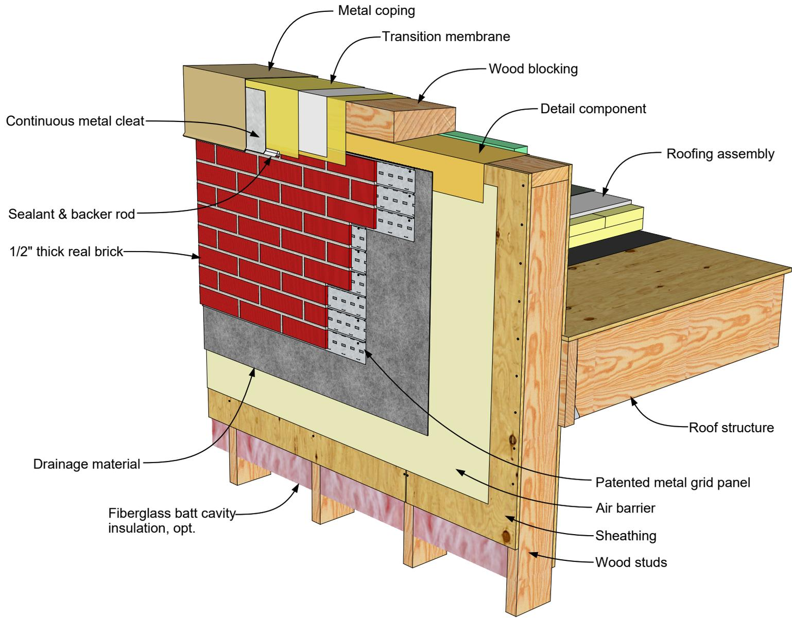
MCS Exterior Wall, Wood Stud Backing | Top of Wall
