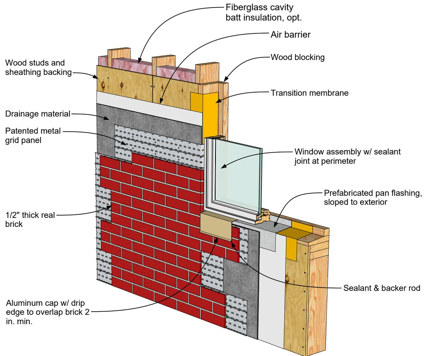
MCS Exterior Wall, Wood Stud Backing | Window Sill
