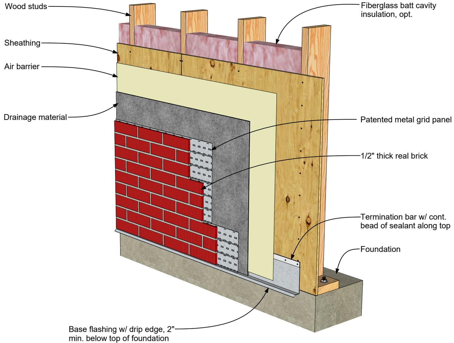
MCS Exterior Wall, Wood Stud Backing | Base of Wall
